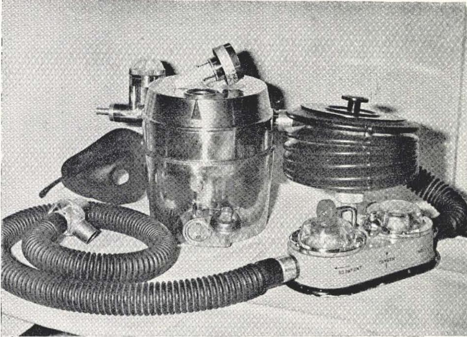
Figure 1. The Gardner Universal Vaporizer with Halothane control unit removed and resting on top of the apparatus.
