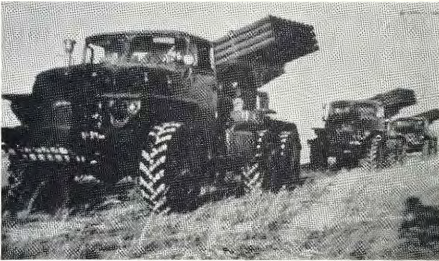
Fig. 1. The multi-barrelled rocket launcher, or "Stalin Organ," is regarded by the Soviets as a psychological weapon to shock, paralyze, daze and stupefy rather than kill or injure. One battery can deliver 720 rounds of 122 mm calibre in 30 seconds.
