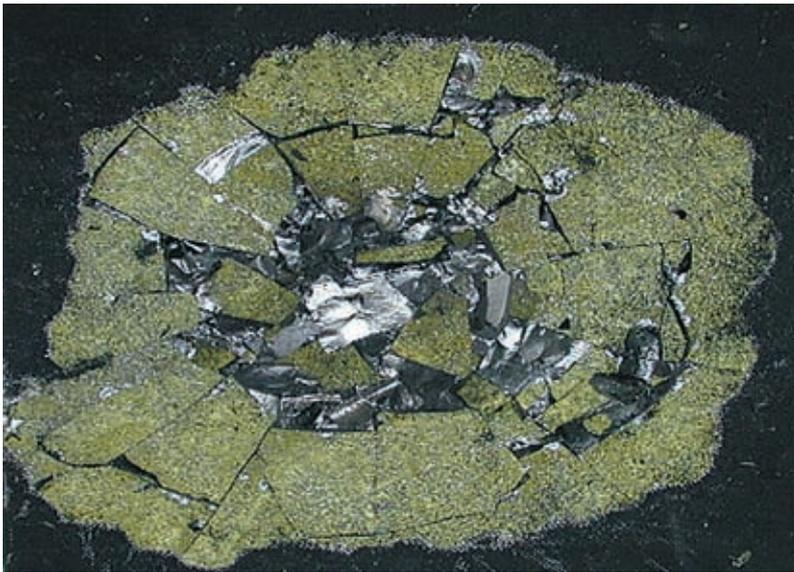
Fig 2. The brittle fracture on the impact face of a boron carbide plate (the black aramid spall shield has been removed).
