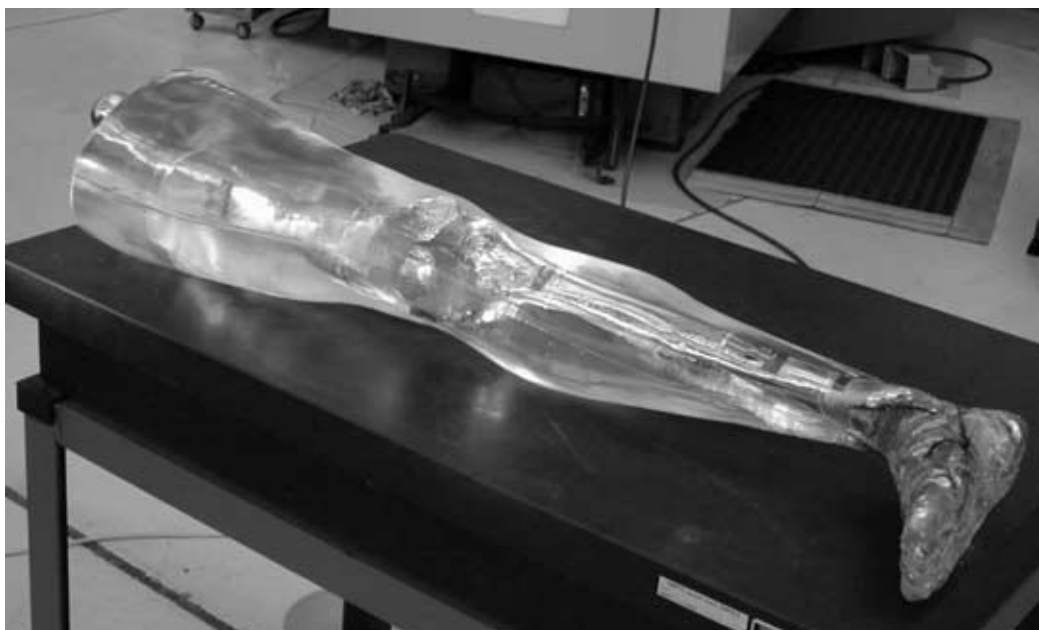
Fig 2. The Frangible Synthetic Leg (FSL). (Courtesy of the Defence Science and Technology Organisation, Australia).
