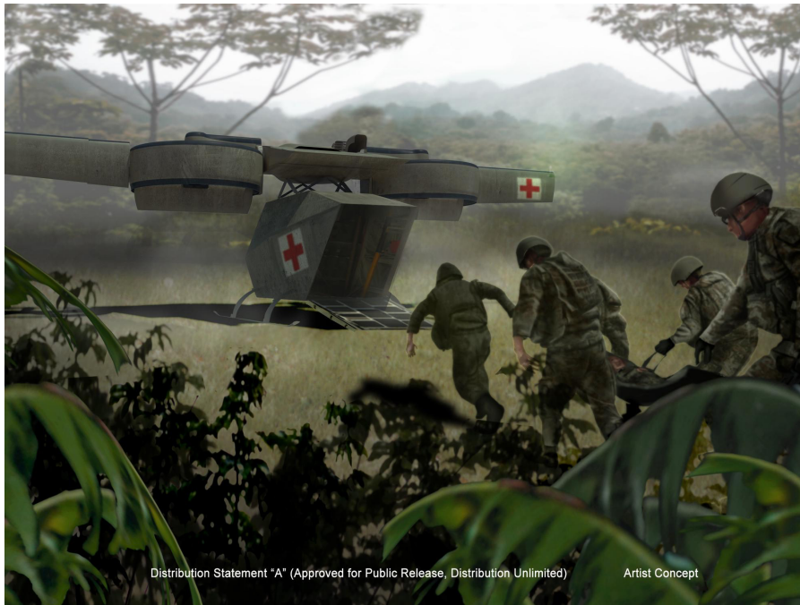
Figure 1 A UAV lands in an austere location to remotely extract a casualty. Aerial reconfigurable embedded system (ARES) medical evacuation module artistic impression by Lockheed Martin. Reproduced with permission from Lockheed Martin.
