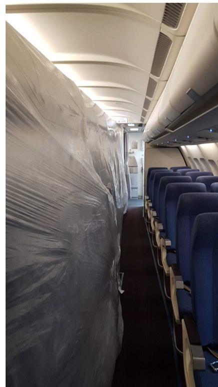
**Figure 1** The aircraft was divided into sections using simple plastic sheeting, erected by the airline ground crew.
