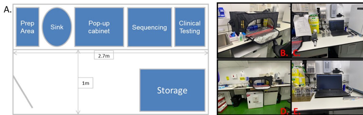
Figure 1 Laboratory design for SARS-CoV-2 WGS aboard RFA ARGUS. (A) Schematic diagram of the laboratory location, with approximate measurements of available space, illustrating the challenging setting for use to provide this complex workflow in a deployable and adaptable setting. (B) Pop-up hood used for sample processing to prevent contamination and enable easy decontamination to take place. (C) Sequencing and amplification equipment set-up for use. (D) Wide-angle image of the available bench space and limited storage. (E) MinION Mk1B and laptop. RFA, Royal Fleet Auxiliary; WGS, whole genome sequencing.
